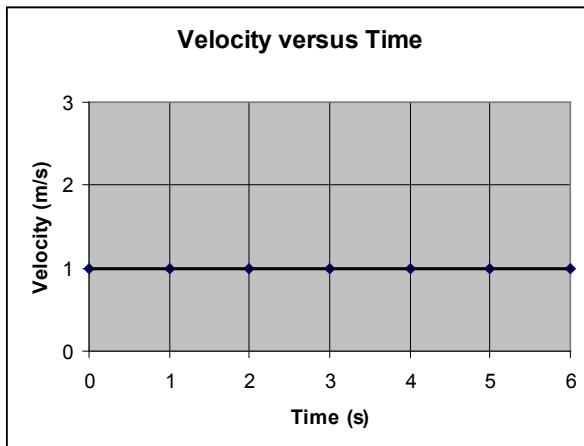
In this case, the object's velocity can be read directly off the graph, but its displacement and the distance it has traveled cannot. However, we can determine the object's displacement, how far it is from where it started, and the distance it has traveled by measuring the area under the curve (in this case the horizontal line at  $v = 1 \text{ m/s}$ ). (If the velocity is always positive, the distance traveled and displacement will be the same.)
