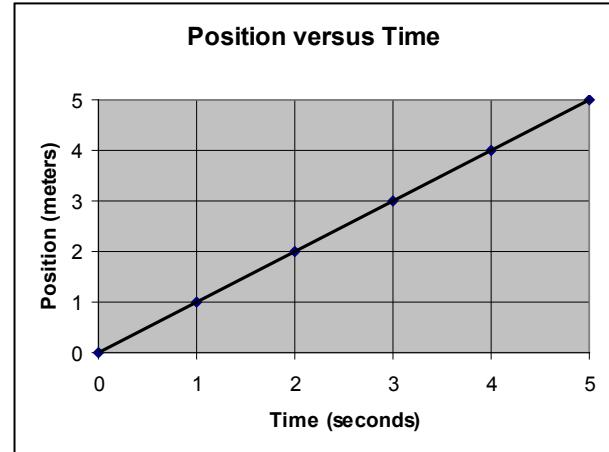
You can also indirectly read your velocity from this chart. **The velocity of an object will be the slope of the line on its Position versus Time graph.**
