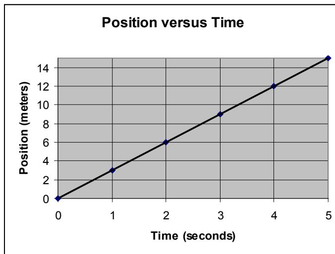
Solution: The location of the object can be read directly off the graph by noting that when the time is equal to  $2.5\text{s}$  then the position is equal to 7 meters. The velocity is constant during the entire trip (hence the straight line) and so it can be found by determining the slope of that line between any two points. Usually we pick points that are easy to read and are as far apart as possible. In this case, let's use the points  $(0,0)$  and  $(4,12)$ .
