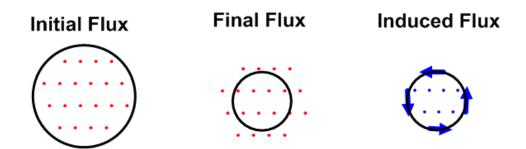
The arrows drawn in the last drawing illustrate that a counterclockwise (CCW) current would be induced.
