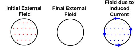
the arrows drawn in the last drawing illustrate that a counterclockwise (CCW) current would be induced.
