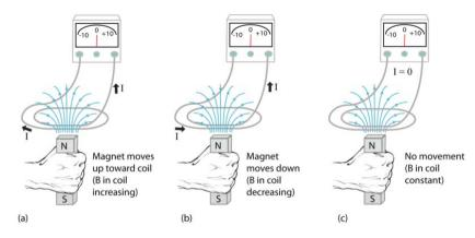
true if the south pole approaches the coil, but the field, and flux, will be in the opposite direction.
