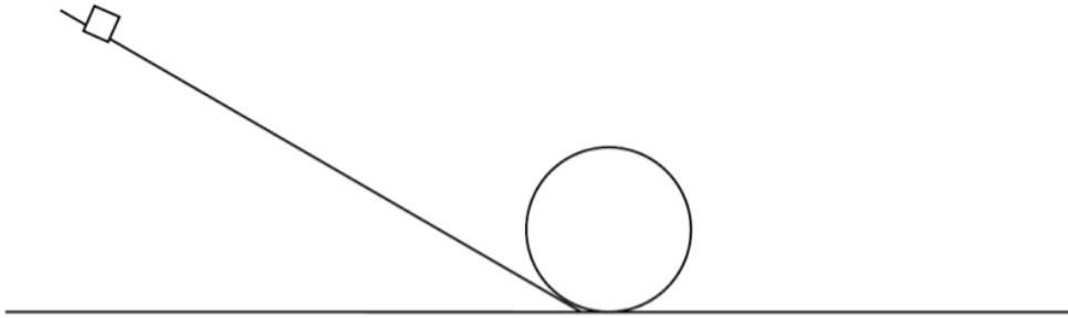
94. A small block, with a mass of 250 g, starts from rest at the top of the apparatus shown above. It then slides without friction down the incline, around the loop and then onto the final level section on the right. The maximum height of the incline is 80 cm, and the radius of the loop is 15 cm.
