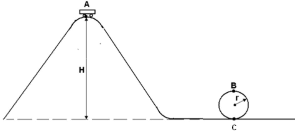
99. A roller coaster of mass 500 kg starts its ride from rest at point A. Point A is located at a height of 70 m above the lowest point on the track. The car rolls down the incline and follows the track around a loop of radius 15 m. Ignore friction force.
