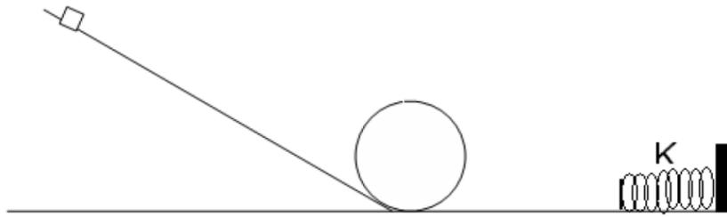
98. A small block, with a mass of 1.5 kg, starts from rest at the top of the apparatus shown above. It then slides without friction down the incline, around the loop and then onto the final level section on the right. It then collides with a spring which momentarily brings the block to a stop. The maximum height of the incline is 2.5 m, the radius of the loop is 0.9 m and the spring constant is 90 N/m.
